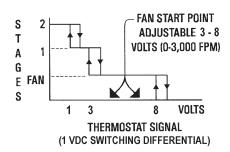
NOTE: There is a 1 VDC switching differential on each stage.
