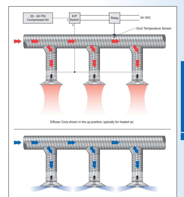
Diffuser Core shown in the down position, typically for cold air.
