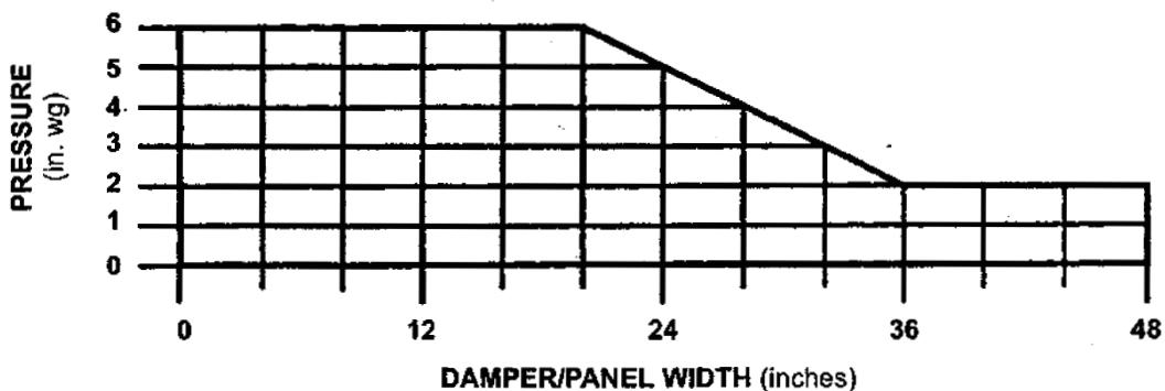
Leakage and differential pressure torque will increase with increased pressure, therefore, adjustments must be made when determining leakage and/or the actuator requirements for a damper. The following table gives multipliers for increased pressure applications.
