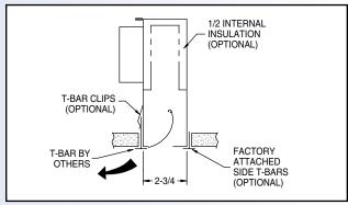
Model FSR-L - Supply / Return, Lay-In T-Bar
