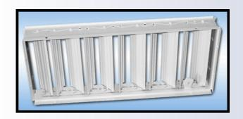
As a general rule, adding an opposed blade damper to a supply or return grille or diffuser with the damper blades set to 100% open will increase the NC by appoximately 3-4 NC and increase in the static pressure (Ps) by about 20%. Because the purpose of using a damper is to balance the airflow to the design CFM required for the outlet, the damper blades will typically be rotated to some position less than 100% open.
