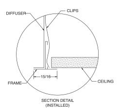
AUXILIARY FRAME SNAPS ONTO INSTALLED DIFFUSER
